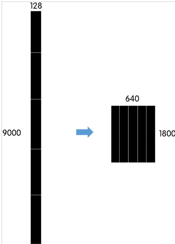
When you set the connection of receiving cards and an Ethernet port loads two rows/columns or more, the connection must follow the shape of the letter Z, as shown in Figure 3-6 and Figure 3-7.
